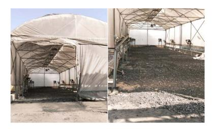
The initial moisture content of the wet sludge was 82%, however on the fourth day the final moisture content of the sludge was reduced to just 20%.
